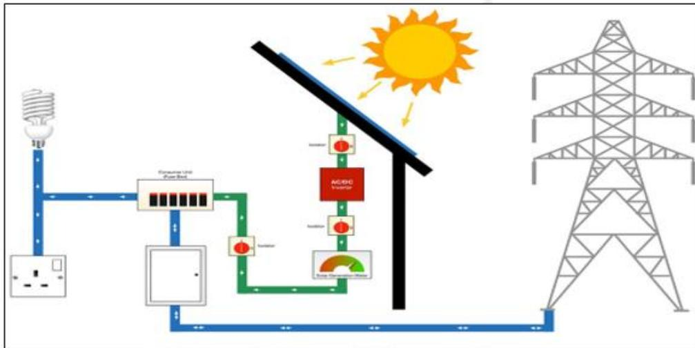
Figure 6: Example Diagram of Solar PV Layout
